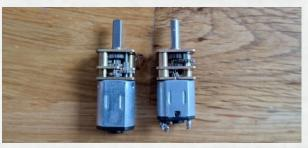
In the picture above you can see the two models, on the left the N20 engine and on the right the N10. The few millimetres in size already make a big difference for the model and the implementation. To check this in advance, I made a cube the size of the motor in MS 3D Builder and sunk it into the 3D model to see if it would fit and with the N10 it would. More on this later in the article.
