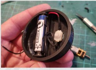
After everything was wired up, I put the heat-shrink tubing over the cables and then soldered the motor on. Incidentally, you don't necessarily need to pay attention to the correct poles here, as this only changes the direction in which the motor turns.
