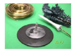
Apply super glue to threads and shaft of screw and screw the large end of the golf tee onto it to contact the topside of the small
